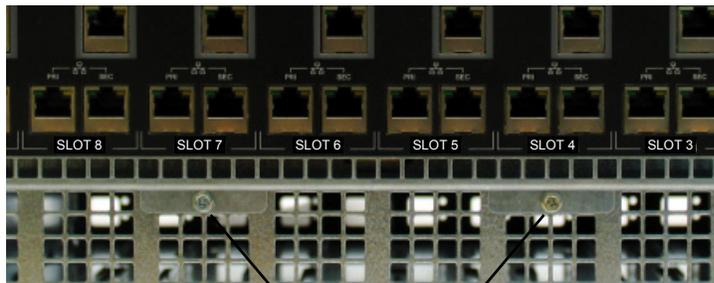
Insert both screws into backplane flanges
