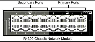
**Video Host card with PCoIP® technology:** For blades with this video configuration, the primary port is Gigabit Ethernet and the secondary port is for PCoIP communication. For example, if the blade is in slot 3, primary port 3 provides Gigabit Ethernet and secondary port 3 provides PCoIP communication.
