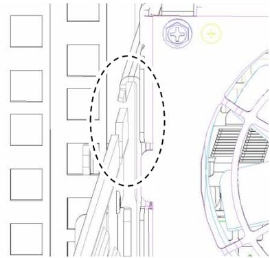
6. By pushing on the front of the Chassis, slide the Chassis Brackets onto the Rack Brackets until the Cage Bracket is flush with front of the Rack.
