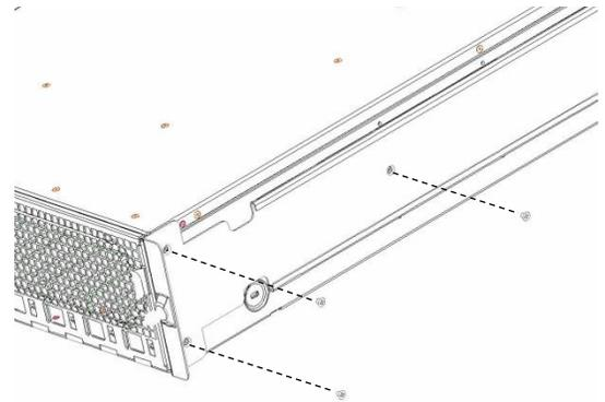
2. Determine the hole locations on the rack that will be used to mount the rack ears on the bracket (use the included alignment guide for assistance). Insert the slider (back) rack ears on the bracket into the holes on the rear post of the rack.
