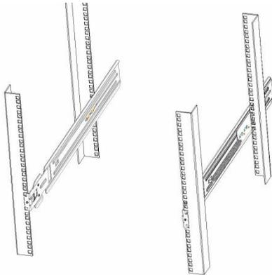
5. Lift the Chassis and align the open "U" channels on the Chassis Brackets with the flanges on the Rack Brackets.
