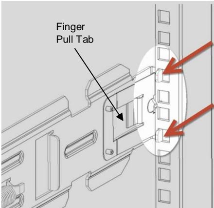
4. Repeat steps 2 and 3 with the other Chassis bracket on the opposite side of rack. Ensure brackets are at the same height with respect to each other.
