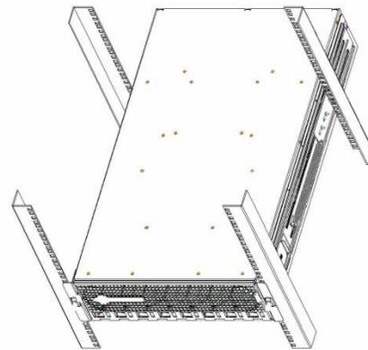
7. Secure the Chassis Bracket to the front of the rack using the thumb screws. Fully tighten them with a Phillips head screwdriver.
