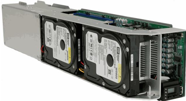
The R2200 dual-Xeon blade offers dual integrated gigabit Ethernet controllers and NVIDIA-based graphics to deliver a high-performance, high-throughput solution to your enterprise computing needs.
