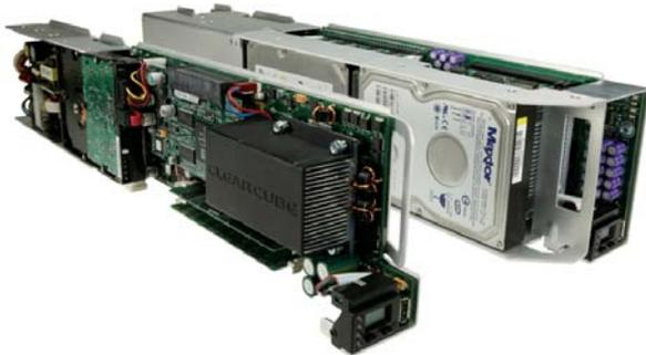
In addition to thermal considerations, the blades must be kept in a relatively clean environment. The electronic circuitry on the blades and chassis modules is not protected from airborne contamination by dust or chemicals. Therefore, the chassis must be kept away from areas with high concentrations of contaminants.
