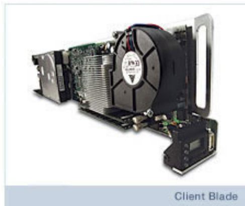
A ClearCube blade contains a CPU and hard drive.
