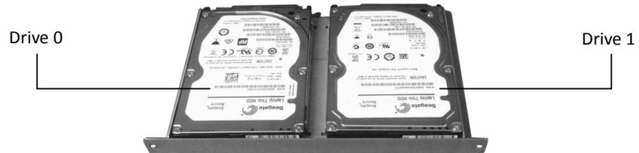
*Figure 4. Drive order in the storage drive carrier*
