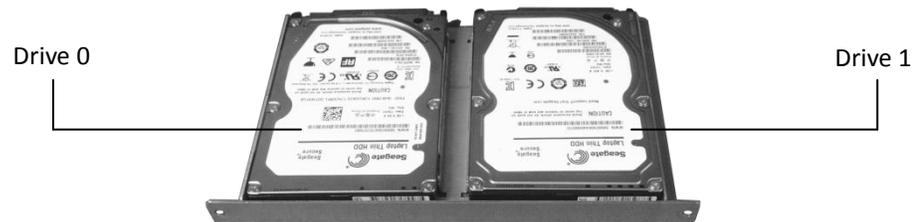
*Figure 4. Drive order in the storage drive carrier*
