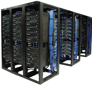
8 Blade PCs 2 PCs per Blade 16 PCs in 3U chassis
